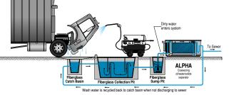
The Alpha can work in conjunction with below-ground catch basins and collection pits or as a stand-alone oil-water separator.
